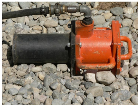
Image 2, pneumatic ram with IPE100 guiding sleeve
